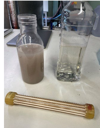
A 1" trial membrane together with the wastewater feed, before and after filtration
