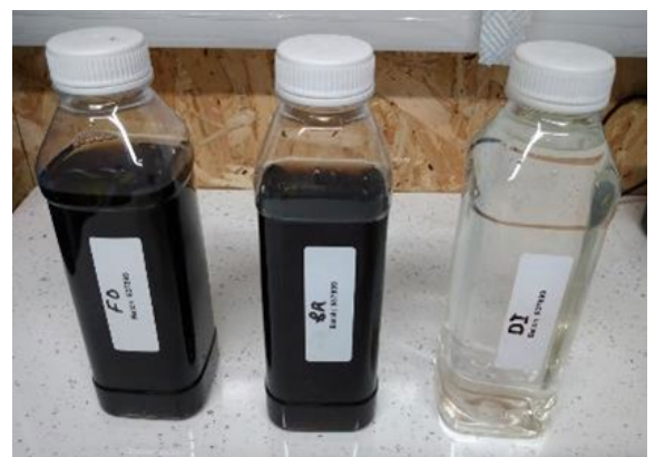
Figure 5 Raw leachate (L), concentrate (C), distillate (R)
