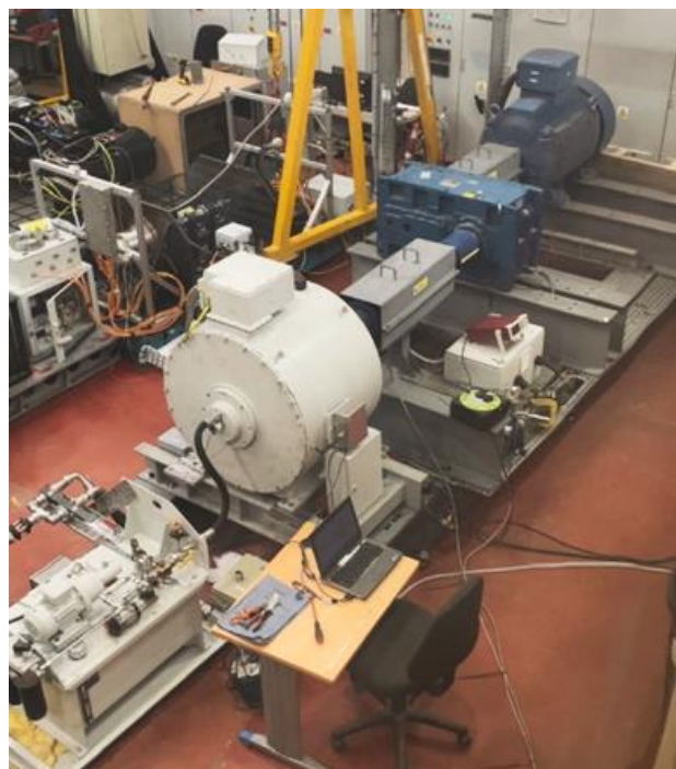
Fig 6. Photo of the dynamometer test-rig at Magnomatics facility in Sheffield during testing
