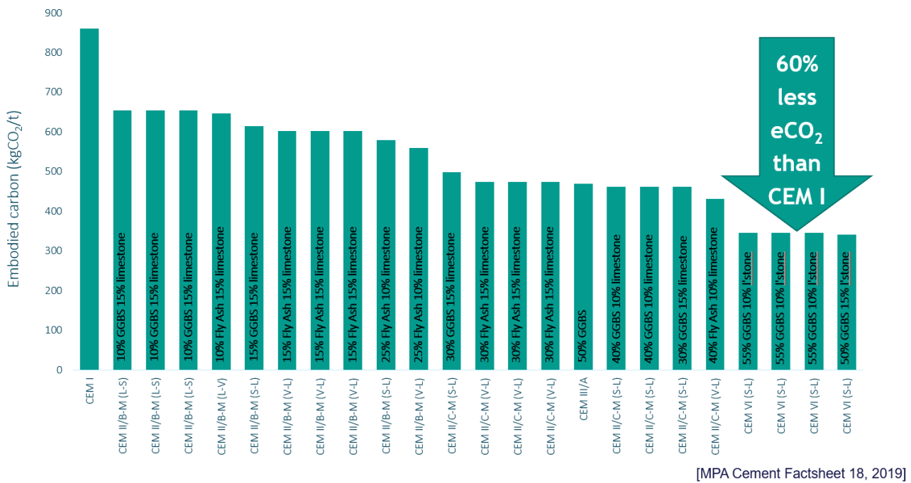
Figure 7 - calculated values of embodied CO 2 of the tested cements versus Portland cement CEM I
