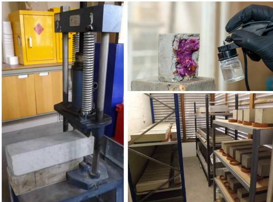
Figure 3 - Photo of the BRE concrete carbonation testing facilities (clockwise from left: splitting the concrete prism, applying indicator solution and sheltered outdoor storage of concrete prisms)
