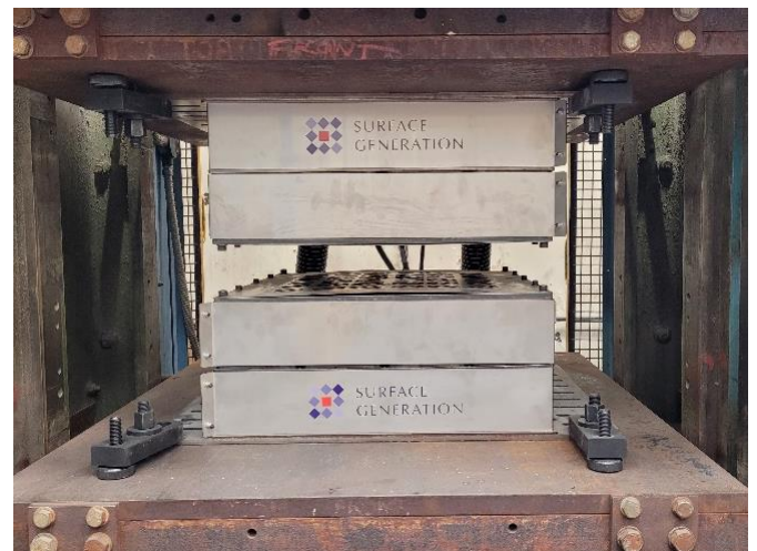
Fig.9, Commissioned PtFS tool installed on press 23
