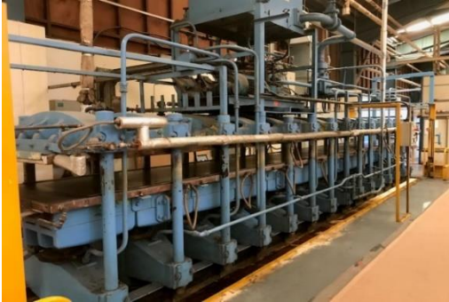
Fig.3, Existing process, compression moulding
